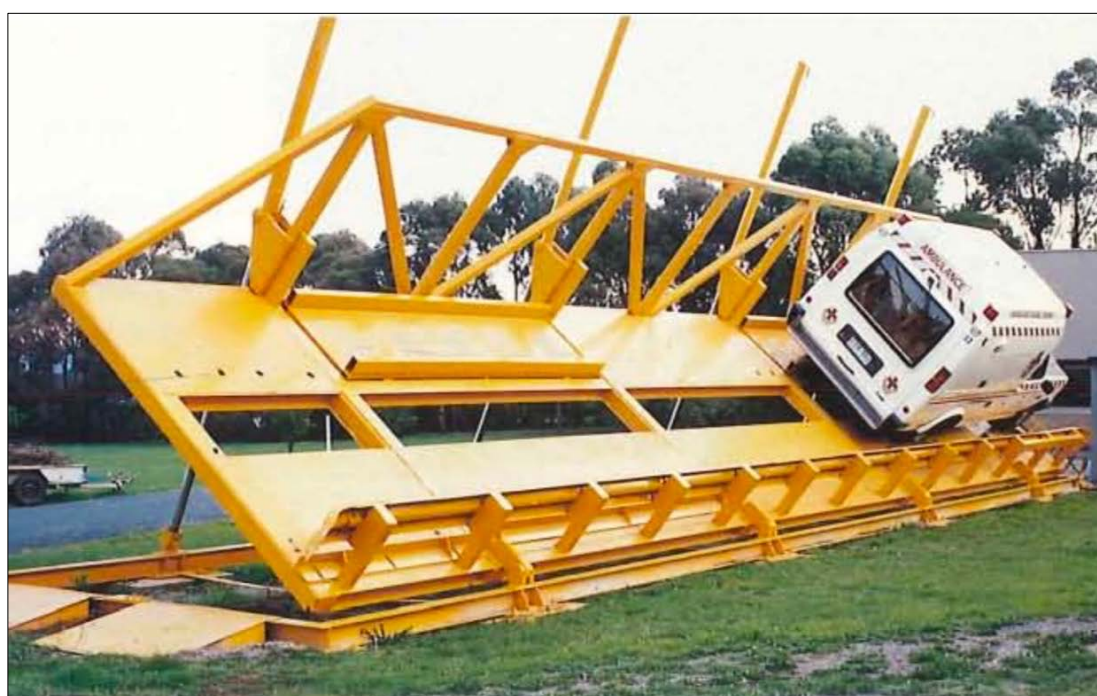
Figure 10 The tilt deck for testing articulated vehicles, installed at the ARRB site in 1984 (removed c2002). Source: ARRB 1993 Annual Report.
