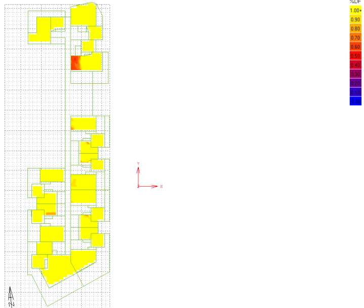
Figure 18: Daylight modelling results for the Level 4 apartments (Building B)
