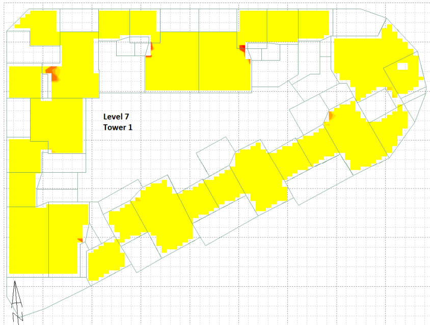
Figure 8: Daylight modelling results for the Level 7 apartments (Building D)
