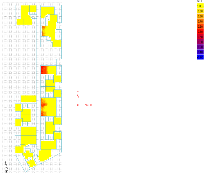
Figure 17: Daylight modelling results for the Level 3 apartments (Building B)
