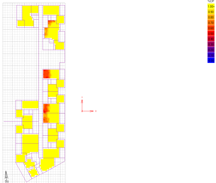
Figure 15: Daylight modelling results for the Level 1 apartments (Building B)
