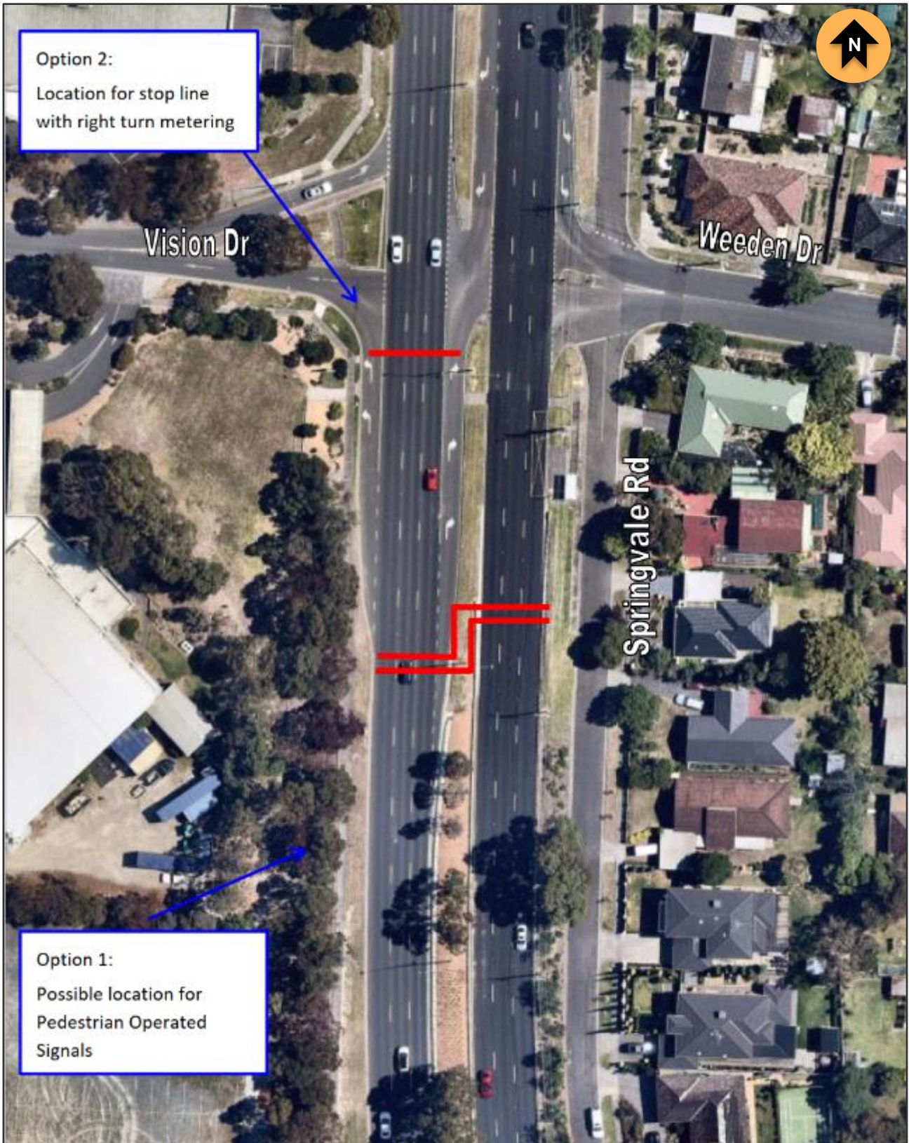
Figure 8 Possible Vision Drive Works
