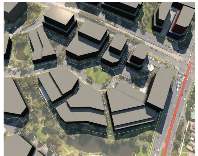
Figure 87 3D modelling and shadow analysis of preliminary revised building heights, subject to further testing for preferred site coverage
