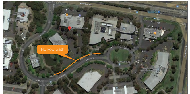
Figure 38 Missing Lakeside Drive northern footpath
